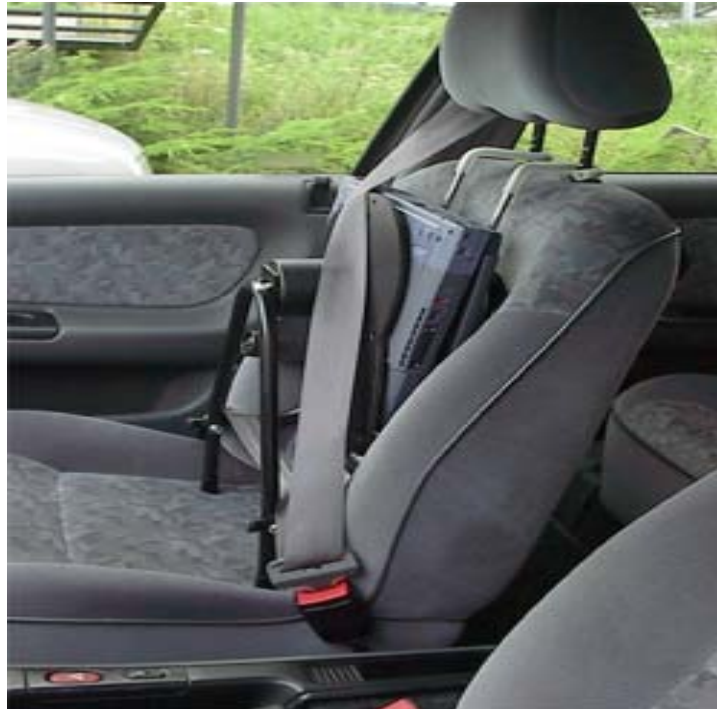
Flip-up CarOffice Portable and secure it with your safety belt if you want to make space on the passenger seat.
